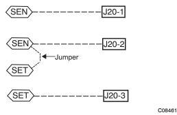
Fig. 62 - RTU-MP T-56 Sensor Connections
